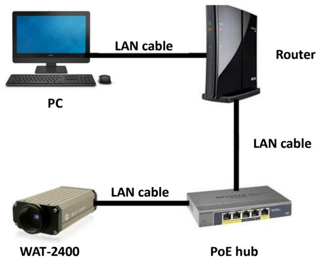
Connect the LAN cable of camera side to a PoE port of the PoE hub and connect the LAN cable of the router side to a normal LAN port.
