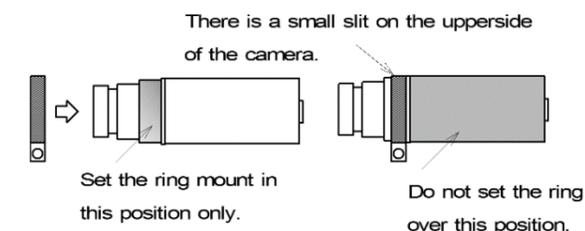
Fix the mount by passing the ring over the lens of the camera, and then attach the thread and nut.
